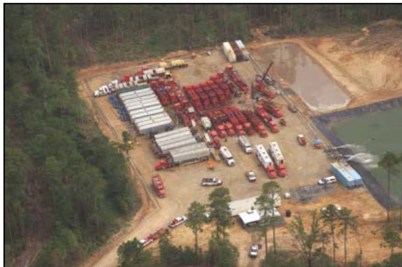
Hydraulic fracturing is a common completion technique in the Barnett shale. Photo from Halliburton.
